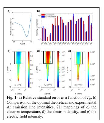
(Fig.1-e). High-resolution 2D mappings of  $T_e$  and  $n_e$  show that the electron temperature peaks at the edges of the plasma jet and decreases towards the center, while the electron density is highest at the jet's core. These trends align with established behaviors of surface-wave plasmas. As for the electric field intensity, it decreases towards the plasma center, with maximum values at the edges, consistent with theoretical and experimental studies of microwave plasmas.
